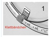
Peel off the cover of the Velcro strip and wrap it overlapping, around the cleaned, dry tube. Du not cut the strip!
